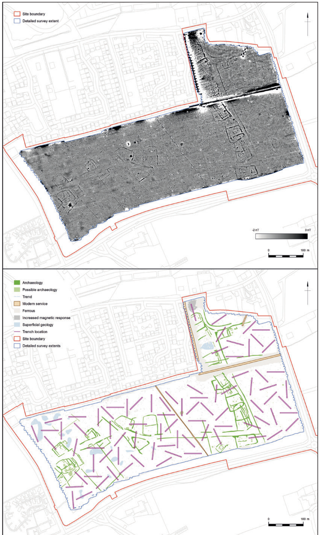
Greyscale plot of magnetic gradiometer survey, illustrating a wide range of archaeological features that can be detected through this technique. Digital data reproduced from Ordnance Survey data. ©Crown Copyright (2020). All rights reserved. Reference Number: 100022432
