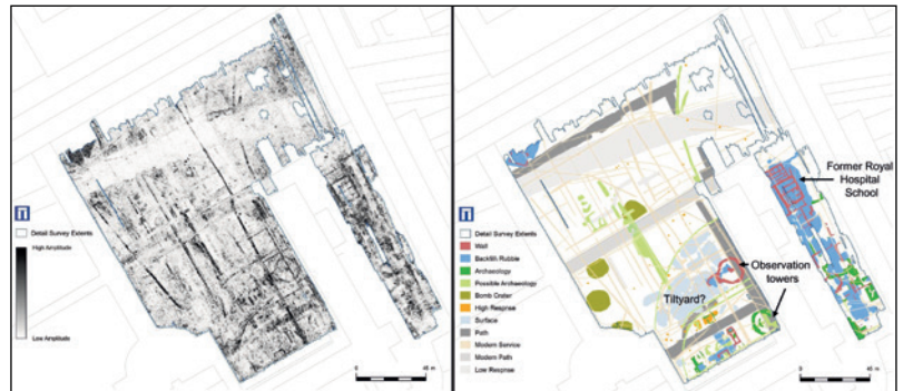
Greyscale plot and interpretation of multi-channel GPR survey from Queen Anne's house in Greenwich, illustrating the location of the observation towers of King Henry's tiltyard. Digital data reproduced from Ordnance Survey data.
