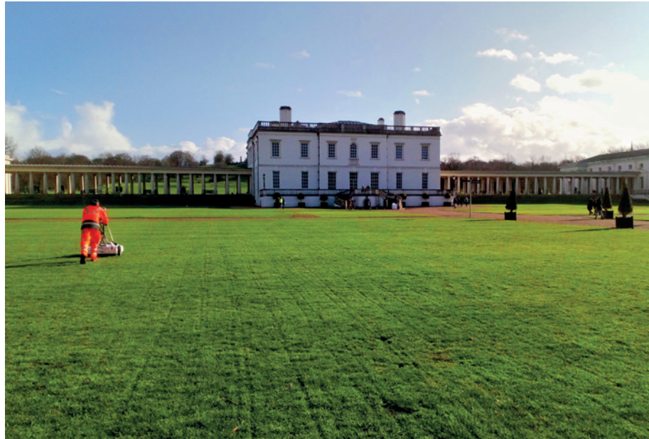
Multi-channel GPR survey in progress at Queen Anne's house in Greenwich, London (NHLE 1002060). The survey was undertaken using an Impulse Radar Raptor array, which contains eight transmitter and receiver antennae spaced 8cm apart, with a central frequency of 450 MHz. Credit: Wessex Archaeology
