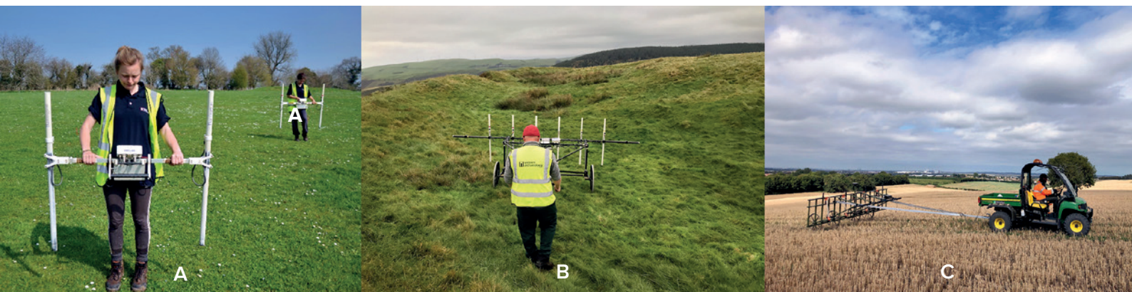
Typical gradiometer setups used in terrestrial geophysics: A) a handheld Bartington Grad601 dual sensor system; B) a non-magnetic cart mounted Bartington Grad-13 sensors; C) an all-terrain vehicle towed array with SenSys FGM650/3 sensors. In optimal conditions, handheld systems allow for approximately 2 ha of survey data to be collected in a single day, whereas cart-based systems and vehicle-towed systems can facilitate more than 5 ha and 10 ha respectively. ©Wessex Archaeology
