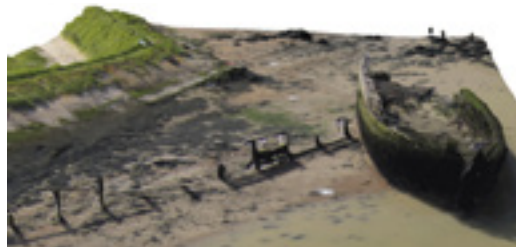
Above: Laying out the targets needed to create a 3D model of the Hans Egede Left: The 3D model of the Hans Egede . Note the dangerous conditions like the height of the tide and the sticking mud that would otherwise mean this could not be surveyed. (Photos: CITIZAN)
