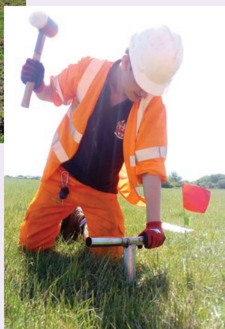
Hammering in an augur for extracting a sub-surface sample for geochemical analysis and to record the geomorphological sequence (© HS2 Ltd)
