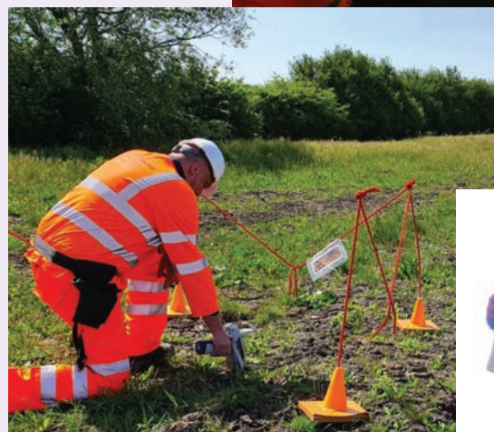
A geochemical sample being taken in the field using the portable XRF machine (© HS2 Ltd)
