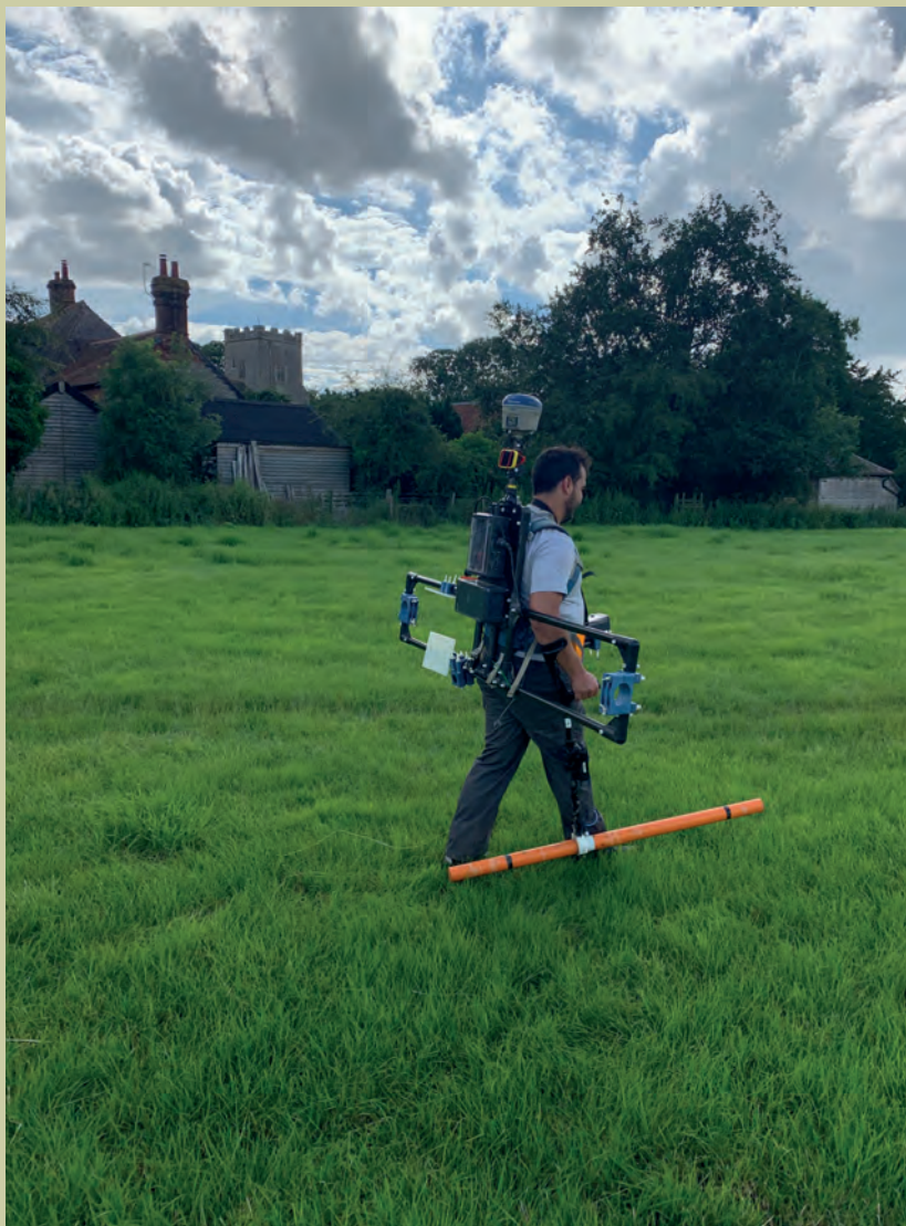
Handheld electromagnetic induction instrument being used to investigate earthworks possibly relating to a medieval manor, Buckinghamshire. Credit: Magnitude Surveys Ltd
