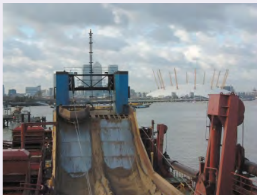
Discharging several thousand tonnes of marine aggregate at Greenwich Wharf, London. Photograph: Mark Dunkley
