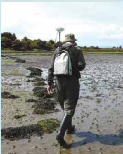
A member of Clyde Shorewatch team plotting a fish-trap in the River Clyde using a GS50 GPS recorder. © CFA
