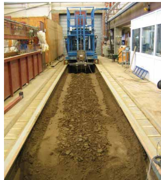
Simulated cultivation in the Cranfield 'soil bin'. © Oxford Archaeology
