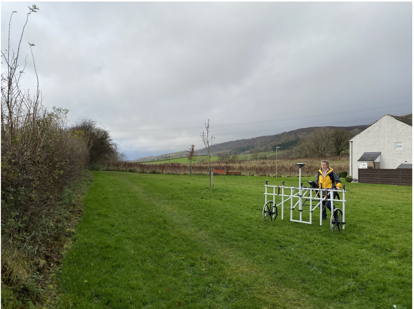
Figure 2: Geophysics team member Hazel Blake operating the Gradiometer at Carleith Farm © HES
