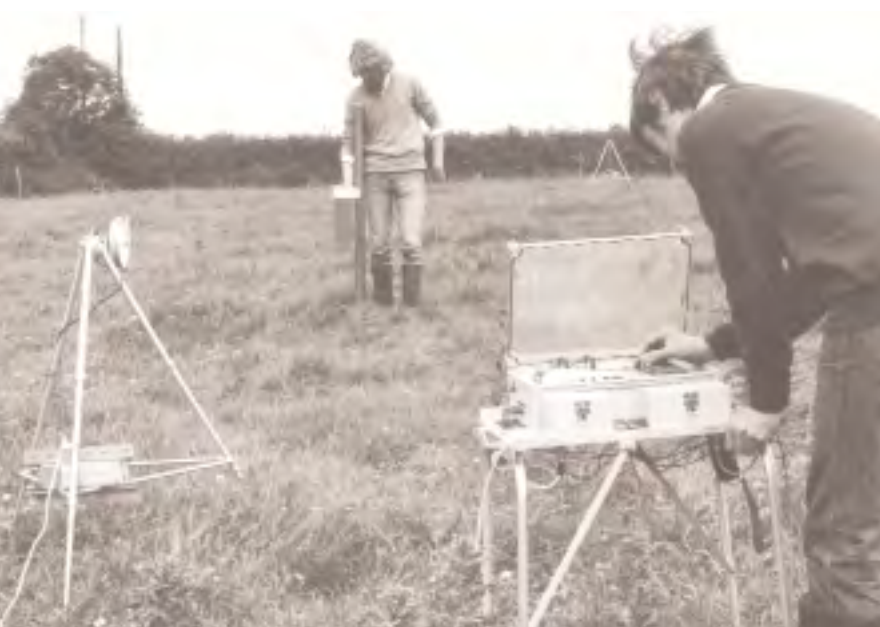
Fluxgate gradiometer and field plotter in use by the Ancient Monuments Laboratory in 1981.
