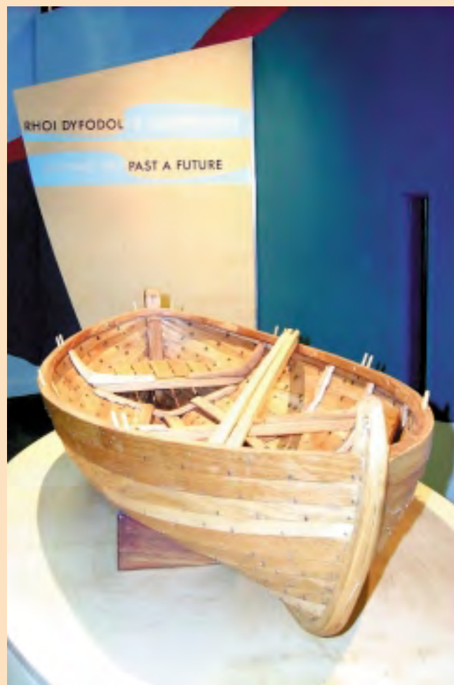
Model of Llyn Peris Boat to showing how it would have looked when first built
