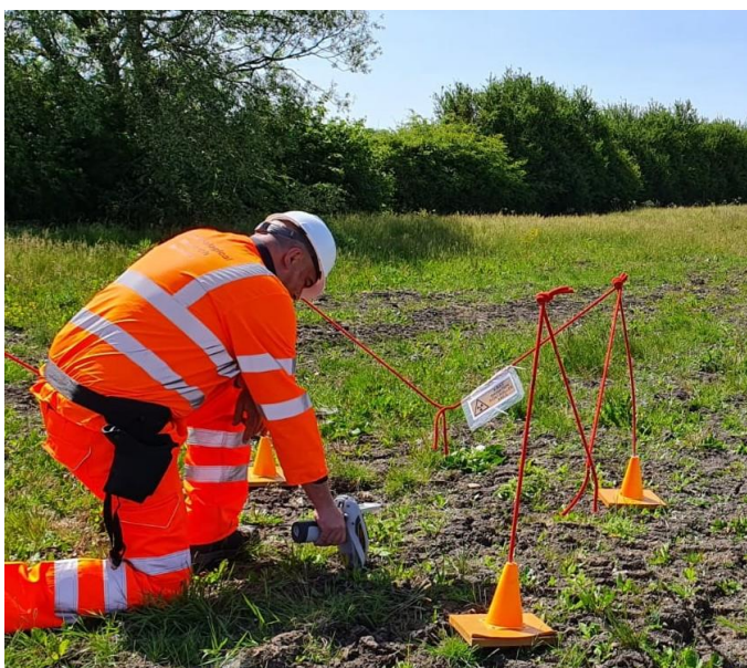
Figure 1 A geochemical sample being taken in the field using the portable XRF machine (© Fusion JV)
