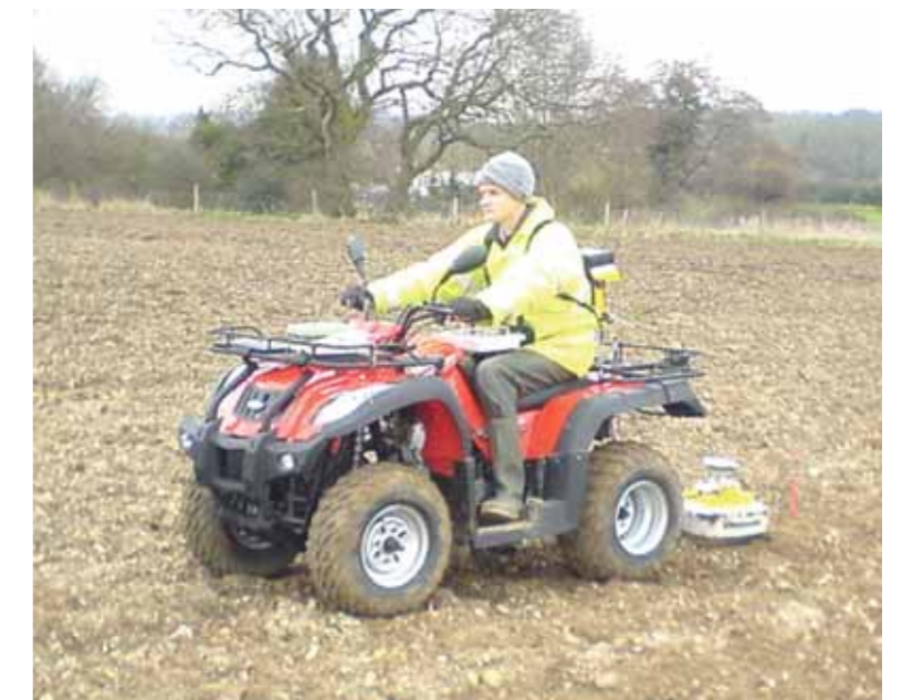
Tim Archer on a 'mechanical horse' (quad bike) which improves survey productivity, while radar is combined with centimetre-accurate GPS. Photograph: Ian Allison
