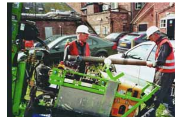
Windowless sampler retrieving sediment cores from backs of burghage plots in Nantwich, July 2007. Photograph: Tim Malim, SLR Consulting
