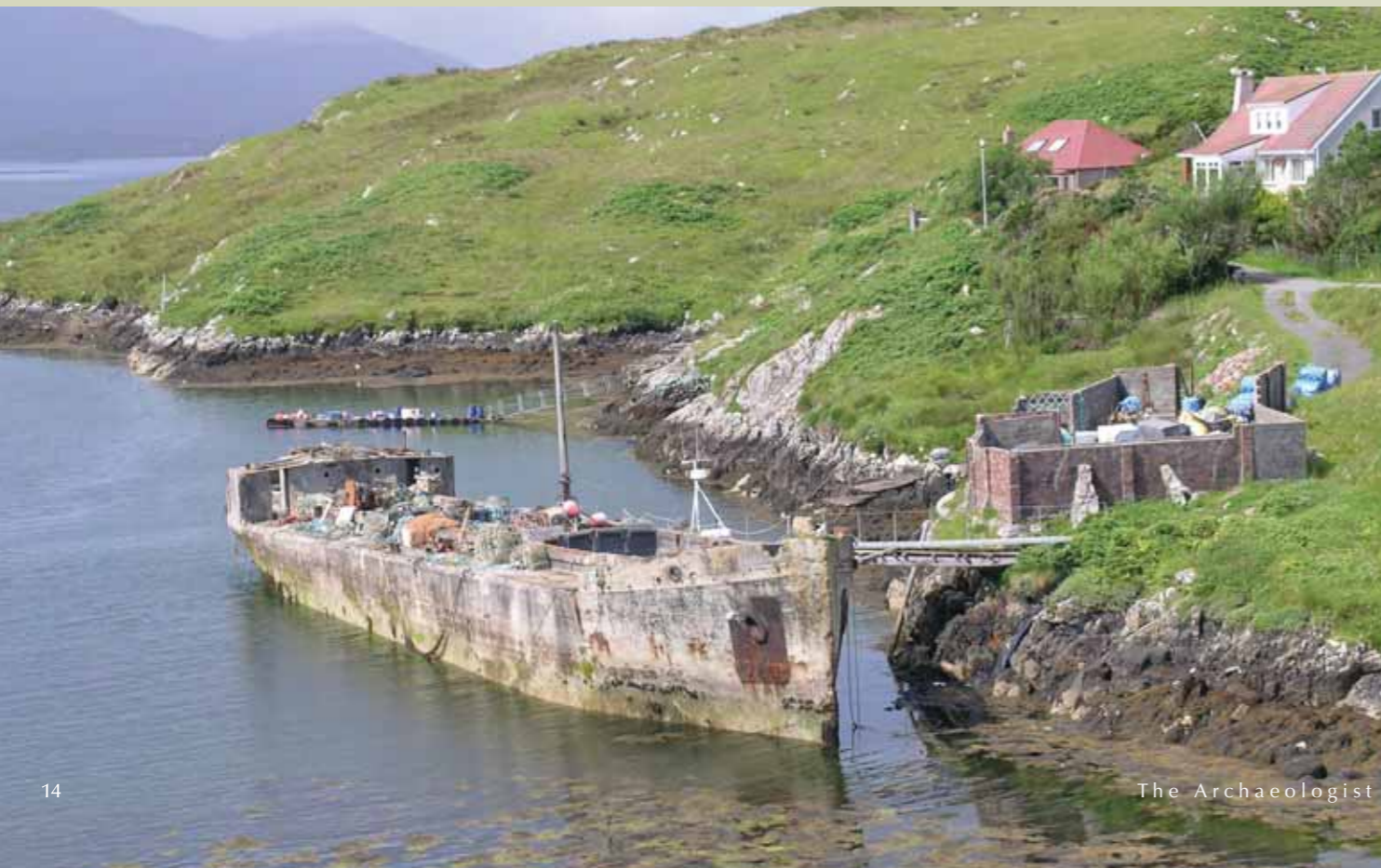
The Cretetree , a collier built of concrete, registered shortly after the First World War and now abandoned
