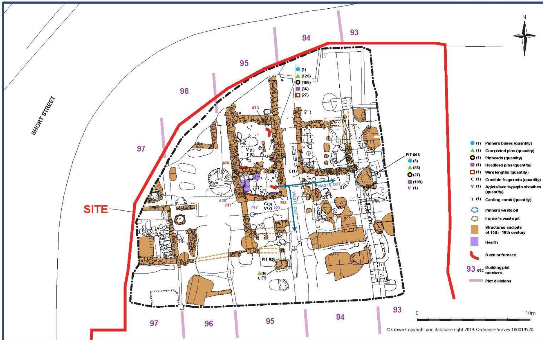
Fig 8: Plan showing the excavated reawing with heat-sources and distribution of pinning debris
