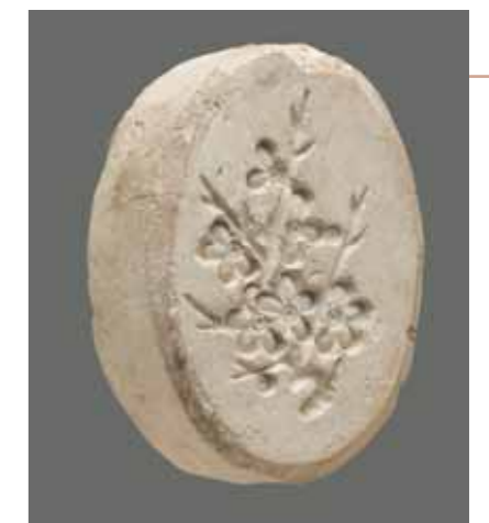
Complete mould for sprigged prunus decoration used on plain white porcelain
