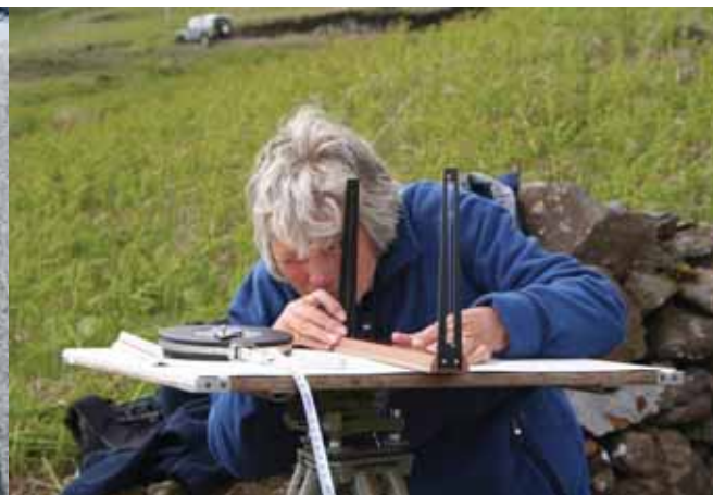
A volunteer using an alidade to record historic rural settlements across Scotland. Crown copyright: RCAHMS
