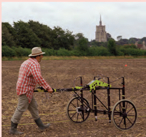
Graeme Spurway using the Foerster magnetometer at Ashwell. Image: Kris Lockyear.
