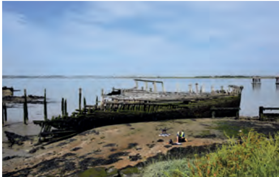
Above: Laying out the targets needed to create a 3D model of the Hans Egede Left: The 3D model of the Hans Egede . Note the dangerous conditions like the height of the tide and the sticking mud that would otherwise mean this could not be surveyed. (Photos: CITiZAN)
