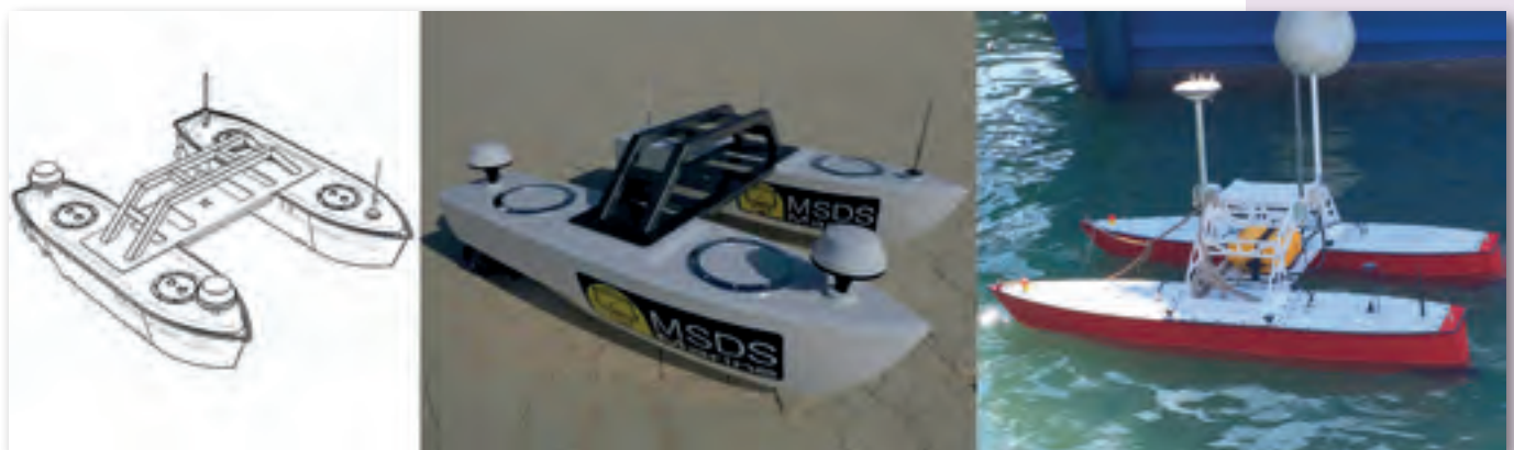
Figure 5: Images showing the work of MSDS Marine and Swathe Services developing unmanned survey vessels, from conception to end product
