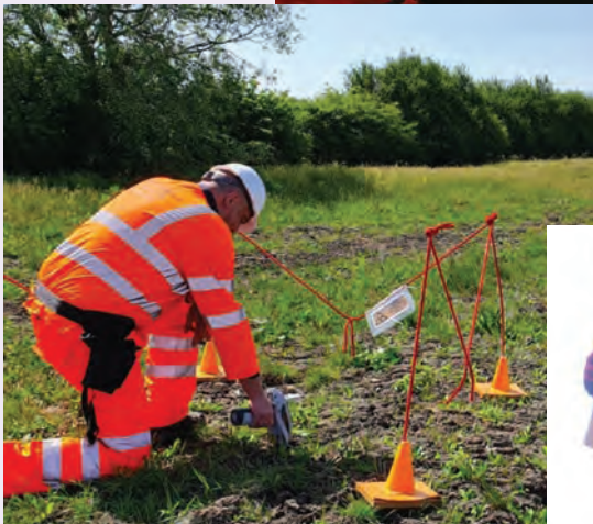
A geochemical sample being taken in the field using the portable XRF machine (© HS2 Ltd)
