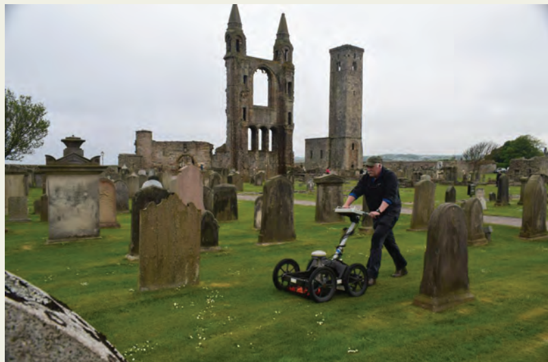
GPR survey being undertaken at St Andrews Cathedral, Fife. Credit: Historic Environment Scotland
