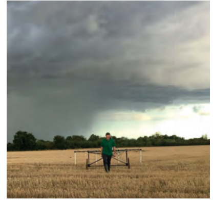
The bespoke Magnitude Surveys' incarnation of the magnetic 'workhorse': four fluxgate sensors with GPS that can be mounted on a hand-pulled cart, carried by hand or towed behind a quad bike, depending on the terrain. Credit: Magnitude Surveys Ltd
