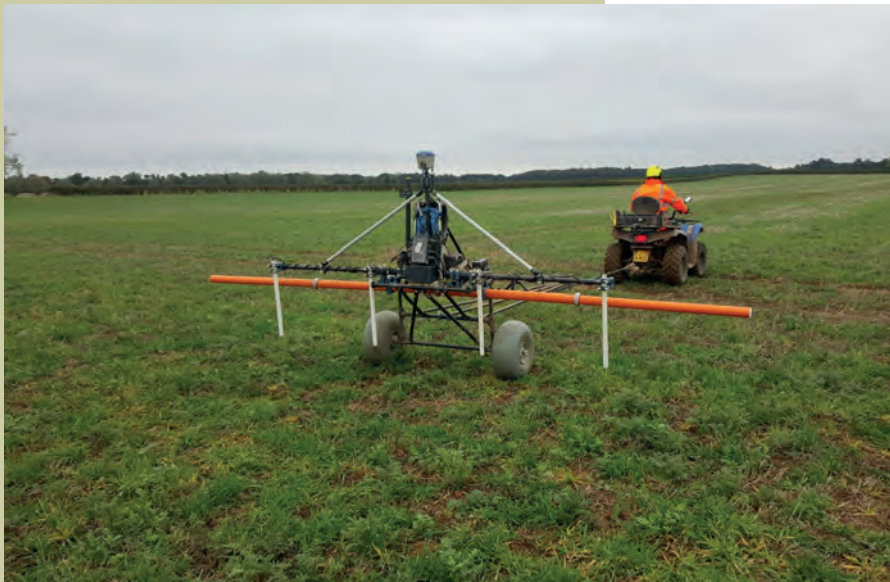
Simultaneous collection of magnetic (vertical white sensors) and EM (horizontal orange sensor) data on a larger scale. Credit: Magnitude Surveys Ltd
