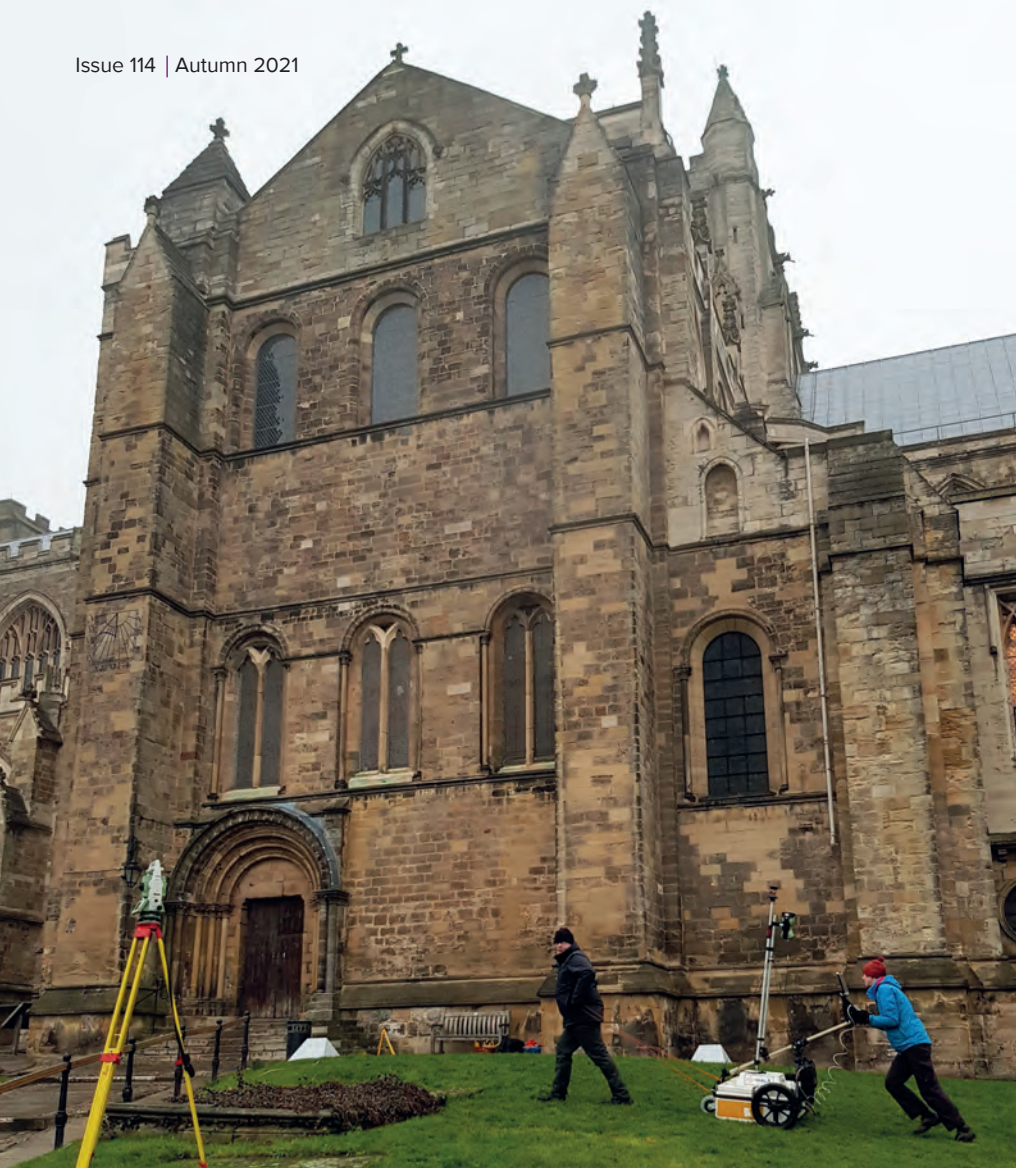
The bespoke Magnitude Surveys' incarnation of the magnetic 'workhorse': four fluxgate sensors with GPS that can be mounted on a hand-pulled cart, carried by hand or towed behind a quad bike, depending on the terrain. Credit: Magnitude Surveys Ltd
