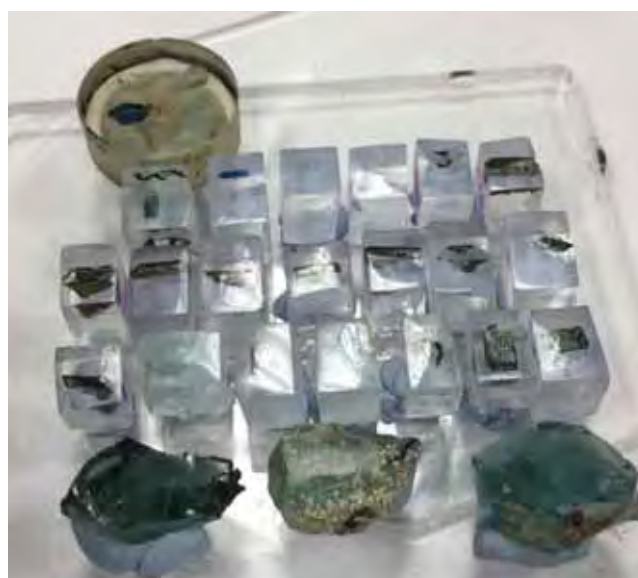
Glass samples mounted and polished ready for analysis by LA-ICP-MS. Credit: Helen Spencer
