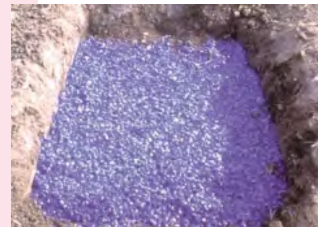
Glass depth disturbance indicators in the plough soil, from The first soil action plan for England: 2004–2006
