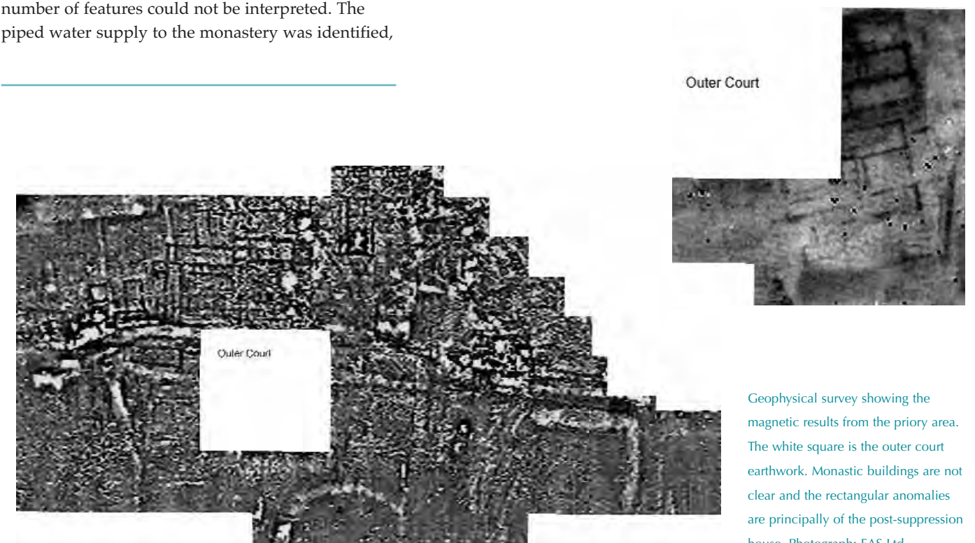
Results of the resistivity survey south and east of the outer court. The east end of the priory church, a chapter house and elements of the west range of the east cloister are clear. Photograph: EAS Ltd
