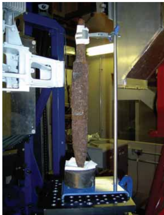
Early Medieval single-edged sword set up for non-destructive analysis on the ENGIN-X diffractometer at the ISIS Neutron Facility, Harwell. Photo: Evelyn Godfrey
