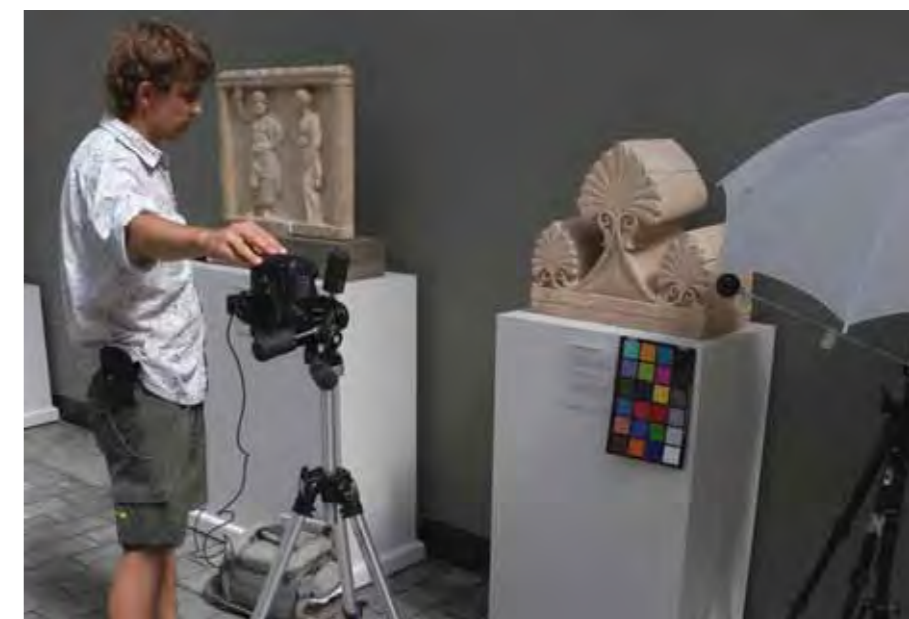
Highlight based RTI: the setup for highlight based capture of small finds. © University of Southampton
