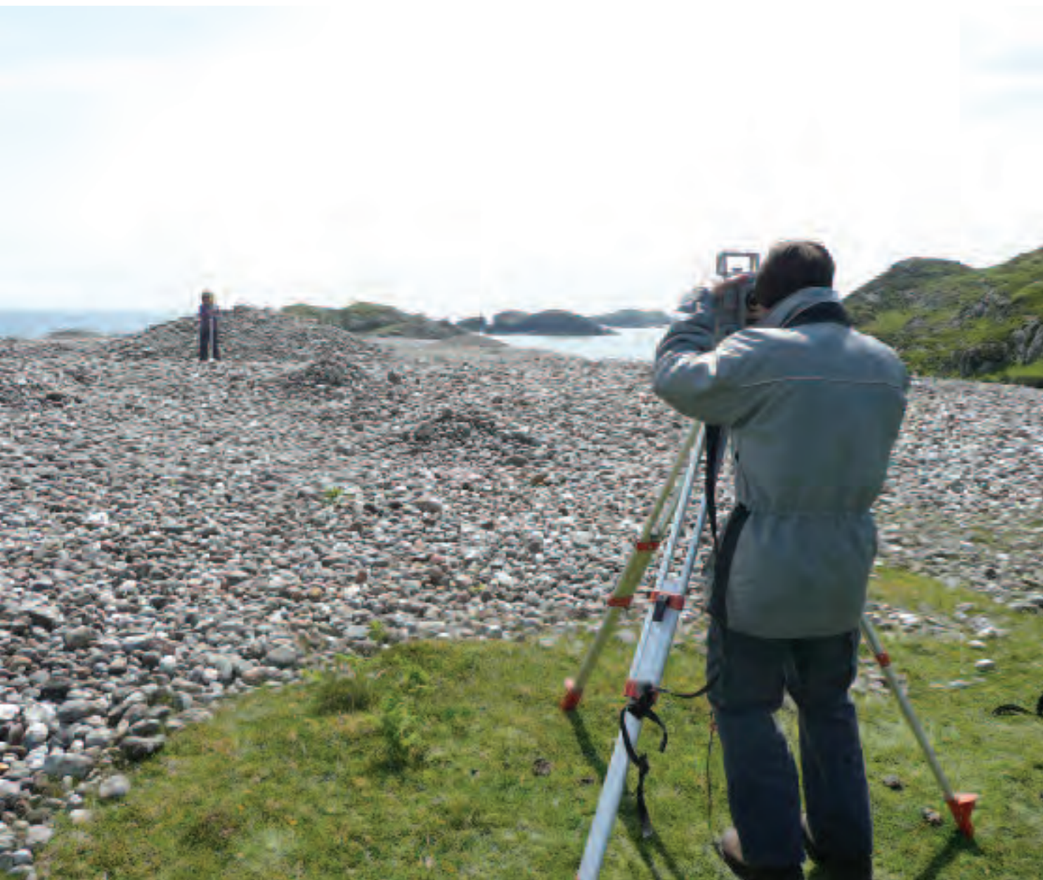
Volunteers using a total station to survey the cairns on Columba's Bay, Iona. © the National Trust for Scotland
