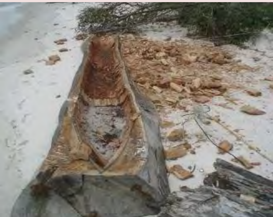
Interdisciplinary studies: traditional crafts and livelihoods – artisanal fishing pirogue under construction, Cap Lopez, Ogooué-Maritime Province, Gabon. © URS
