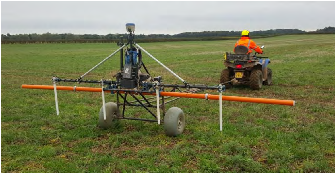
Figure 3.1 Modular cart system simultaneously collecting magnetometer and electromagnetic conductivity data (© Magnitude Surveys)
