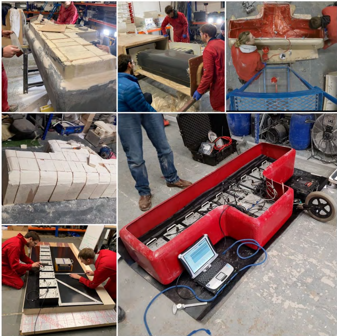
Figure 3.3 The stages of building a bespoke 3D GPR system, starting from the bottom left and moving clockwise: measuring the GPR array to determine the size of the case; assembling a form from CNC-milled MDF and foam; finishing the form surface with polishable primer and resin; curing the first stages of a multi-part mould onto the form using a temperature-controlled cupboard; vacuum infusing resin through the final part in its mould; finished component undergoing initial testing (© Magnitude Surveys)
