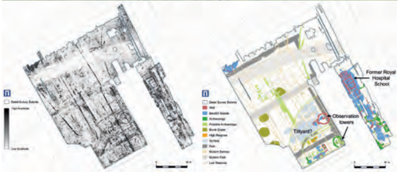
Greyscale plot and interpretation of multi-channel GPR survey from Queen Anne's house in Greenwich Crown copyright (2020) All rights reserved. Reference number 100022432
