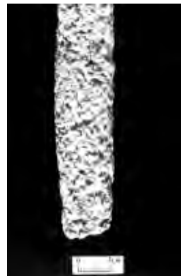
Grade 5+: As grade 5 but with extensive penetrating erosion resulting in modification of profile
